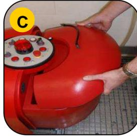
Fill the membrane tank (A) approx. half-way with fresh water. Add the cleaning agent\* (B) and then fill the membrane tank completely to approx. 2cm below the rim. Put the lid on\*\* (C).
